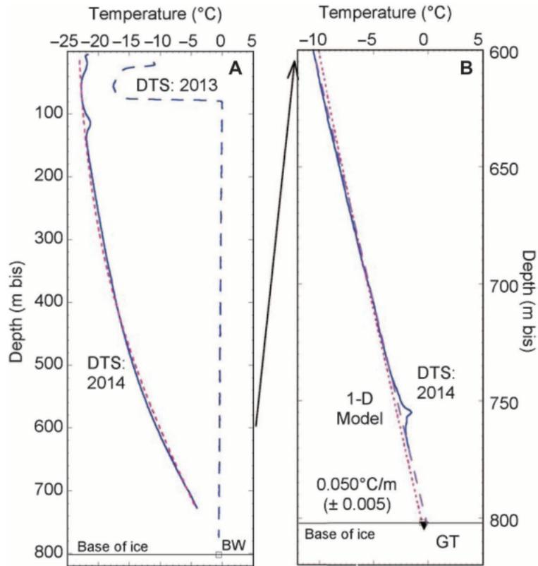
Figure 2: Measuring temperature using distributed temperature sensing (DTS). This graphic is from Figure 3 at Fisher et al. (2015).
