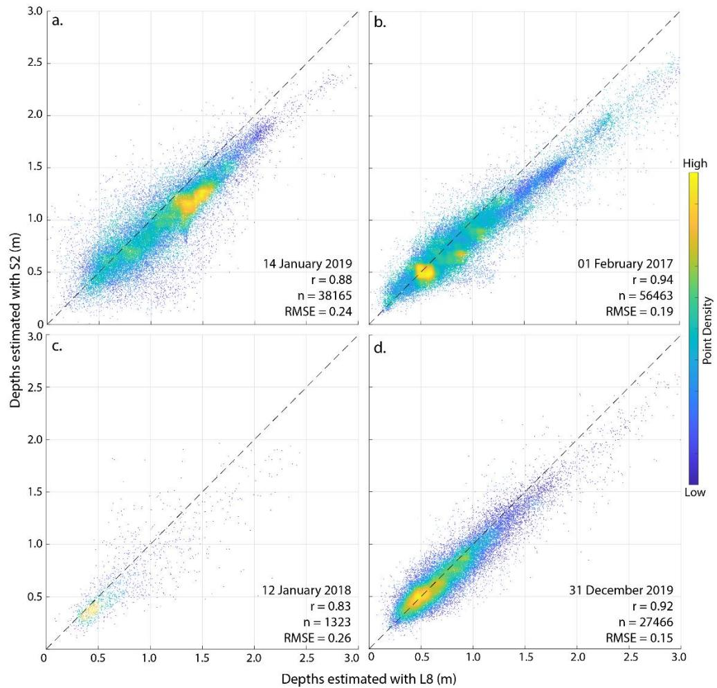
**Figure S1.** Correlation between depths estimated using Landsat-8 and Sentinel-2 products. Each of the plot represents a different pair of Landsat-8 and Sentinel-2, picked from different regions of the study area. The dashed line is the 1:1 line between Landsat-8 and Sentinel-2 depths. The average  $r$  is 0.89 and RMSE is 0.21m.
