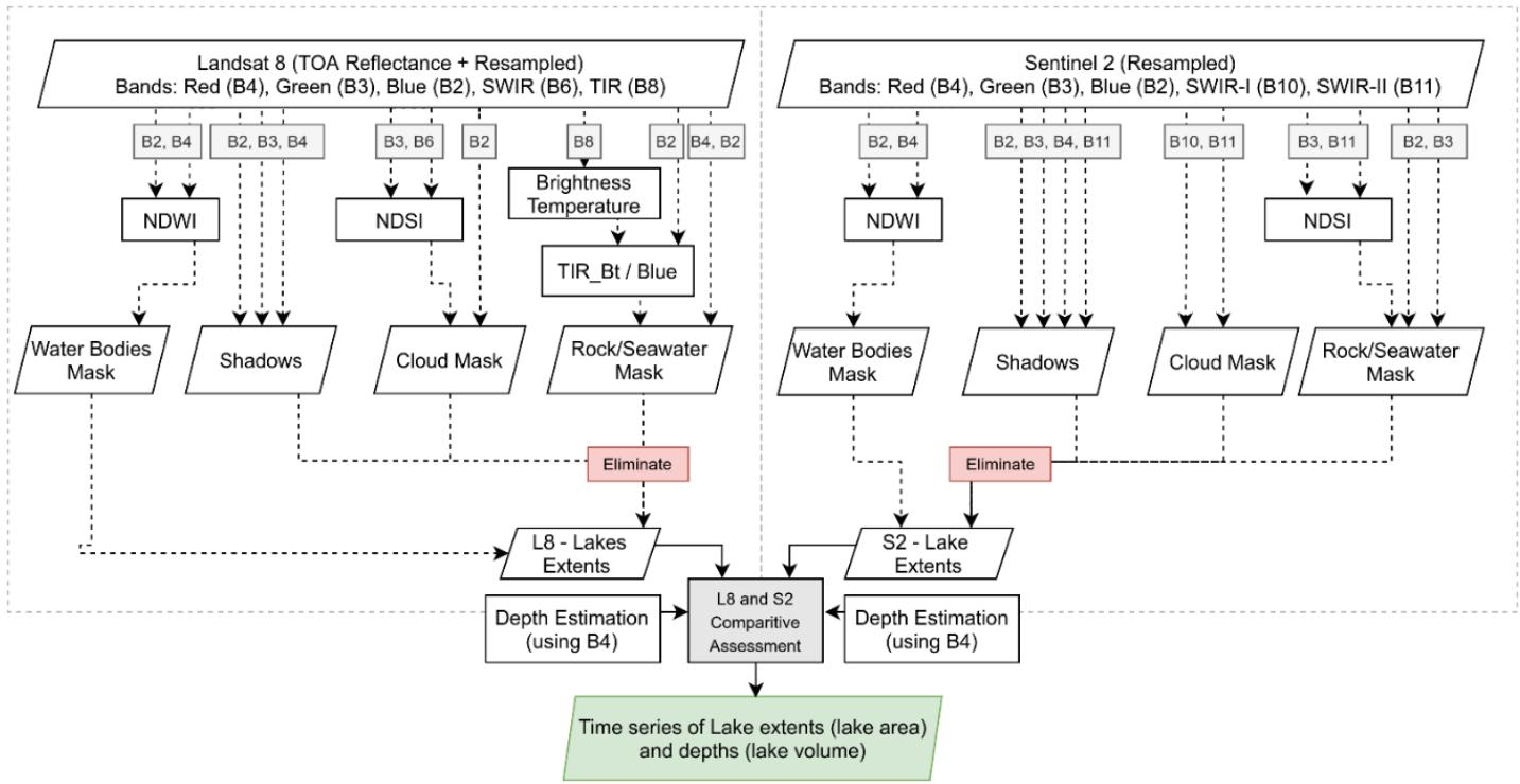
**Figure S7.** Methodological flowchart for automated SGL mapping and depth estimation using Landsat-8 and Sentinel-2 scenes.
