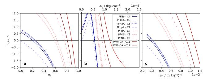
**Figure 1.** Model tuning for each PFAS. The bias, b, was calculated as the sum of the difference between measurements and co-located model layers in three tuning runs. Each panel shows results for a different decoupling method: a) simple decoupling, tuned using  $\alpha_B$ ; b) surface area adsorption, tuned using  $\alpha_C$ ; and c) salinity mediated decoupling, tuned using  $\alpha_D$ . The best performing  $\alpha$  give b closest to 0 (black line).
