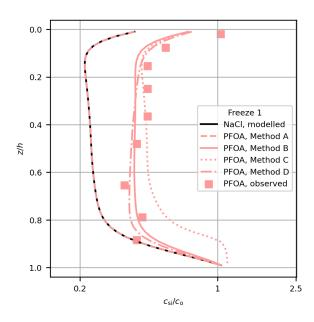
**Figure 3.** Comparison of modelled (lines) and measured (squares) PFOA concentration in Freeze 1 for each method. Modelled NaCl is also shown (black line).
