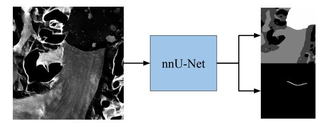
**Figure 1.** Illustration of the modified nnU-Net for simultaneous predicting landscape zones and the glacier front. On the left is an exemplary satellite image of the Crane Glacier taken by TanDEM-X (TDX) on 24 June 2011. On the right, the upper image shows the four segmentation classes: ocean (white), glacier (light grey), rock (dark grey), and no information available (black). The lower image shows the glacier's calving front as a white line versus the black background.
