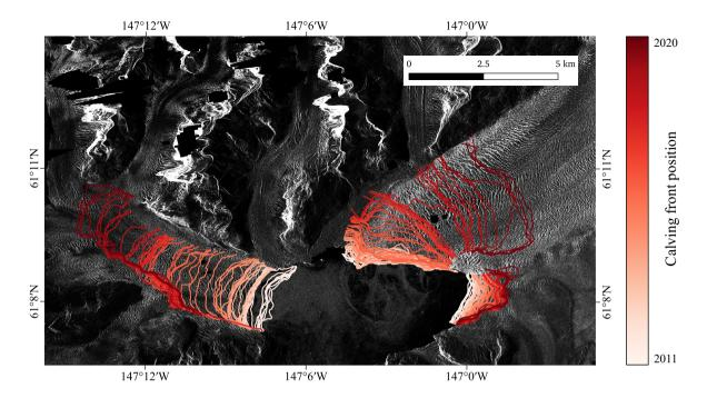
**Figure 4.** Evolution of the calving front position of Columbia Glacier (Alaska). The red lines are all calving front labels available in the dataset. Background: SAR intensity image acquired by TDX on date 13 November 2011. Projection CRS EPSG:4326 - WGS 84 / UTM zone 6N. SAR imagery is provided by DLR, ESA, and ASF.
