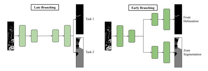
**Figure 7.** Illustration of early- and late-branching U-Net architectures for MTL. Both architectures perform joint feature extraction. The early-branching architecture applies separate reconstruction with two decoders, one for each task. The late-branching network applies joint reconstruction with a common decoder.
