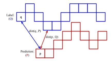
Figure 8. Visualization of the Mean Distance Error (MDE) calculation between front label Q and front prediction P. The dist(q, P) represents the distance between q and the pixel in P that is closest to q.
