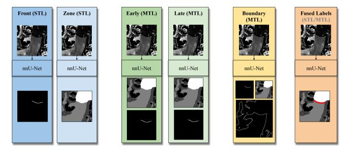
**Figure 6.** Illustration of the six experiments: Two Single-Task-Learning (STL) experiments (blue), two MTL experiments with different architectures (green), one MTL experiment with an additional task of delineating the whole glacier boundary (yellow), and one experiment where the two labels are fused into one segmentation task with an additional class in the zone label (orange).
