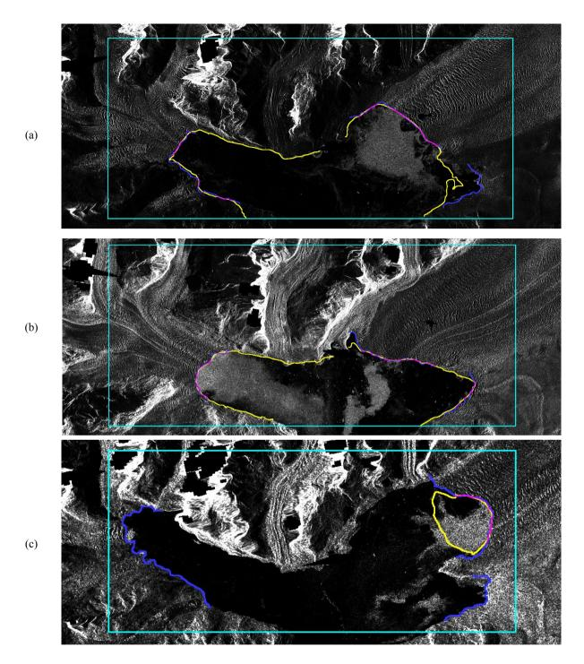
**Figure 13.** Calving front predictions of COL on (a) 11 February 2016, and (b) 22 June 2014 taken by TDX with 7m pixel resolution (after multi-looking with a factor of 3x3); (c) was taken by S1 on 10 September 2019 with 20 m pixel resolution; ground truth (blue), prediction (yellow), the overlap of ground truth and prediction (magenta). SAR imagery is provided by DLR, ESA, and ASF.
