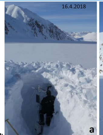
hat gelöscht: Fig. 5: Maintenance of the AWS at Freya Glacier in April 2018: a) The station is 3.5 m tall and was completely covered in snow. b) The weather station and the c) stakes with the second ultrasonic device were reestablished on the snow surface. (Photos: Daniel Binder). ¶
