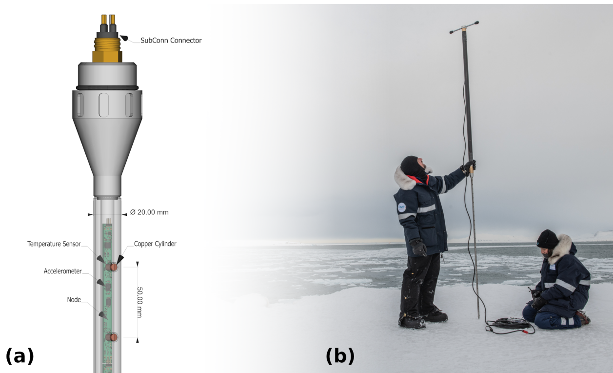
Figure 1. (a) Technical drawing of the head of the temperature lance. A string of 15 nodes is housed inside the lance, with copper cylinders protruding the stainless steel body, coupling the temperature sensors to their surroundings. Two temperature sensors are mounted on each node; on two nodes (at the top and in the middle of the lance) an additional accelerometer is mounted. (b) The temperature lance assembled with one carbon fiber extension for deployment in up to 1.5 m deep water, and connected with a water-proof cable to the logger unit.
