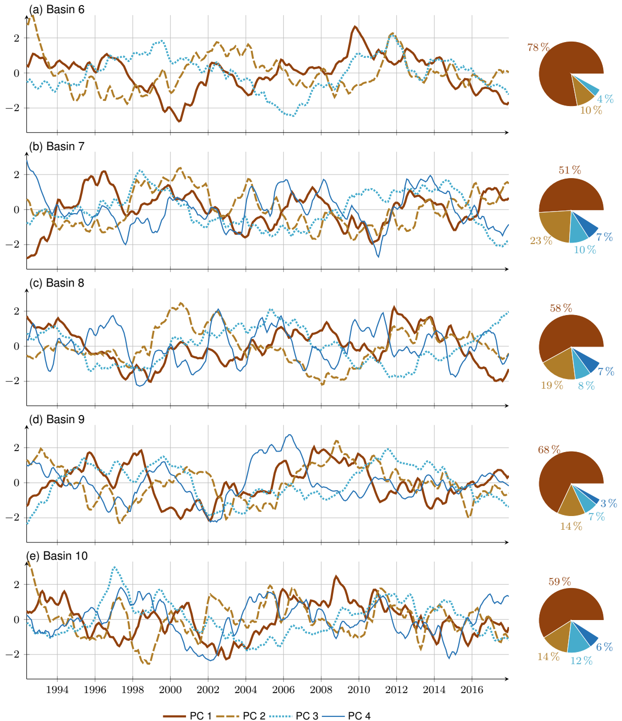
Figure S7. Dominant PCs in firm thickness variations identified by Mb for (a–d) basins 6–10 (line chart) and associated percentages of the basin's total data variance considering the respective PC/EOF pair (pie chart). The respective EOFs are given by Fig. S3 (2nd column).
