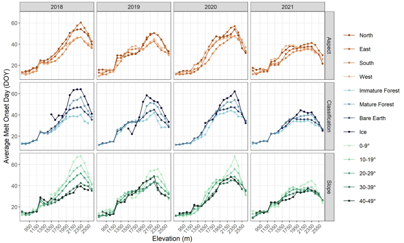
Figure 10. Average estimates of snowmelt duration by elevation, aspect, classification, and slope. Estimates of melt duration are derived from SAR based estimates of melt onset and optical estimates of melt end. Averages are obtained from VV polarized SAR images.
