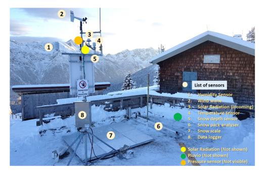
140 Figure 2 Automatic weather and snow measurement station at Brunnenkopfhütte in Ammergauer Alps [1602 m a.s.l.] (Image credit – Wolfgang Bogacki, 2016)
