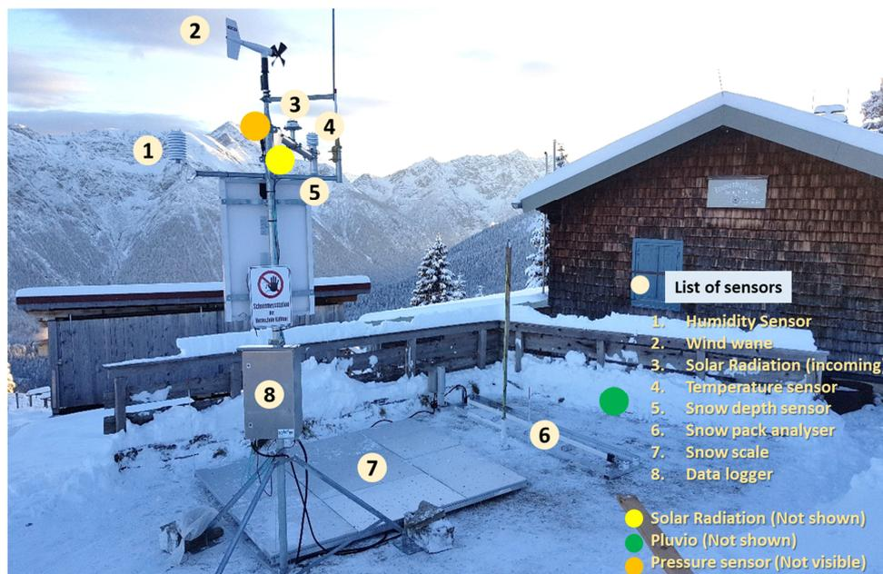
140 Figure 2 Automatic weather and snow measurement station at Brunnenkopfhütte in Ammergauer Alps [1602 m a.s.l.] (Image credit – Wolfgang Bogacki, 2016)
