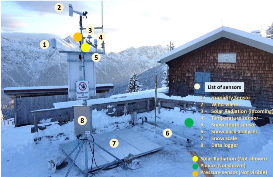
Figure 2 Automatic snow and weather station at Brunnenkopfhütte in Ammergauer Alps [1602 m a.s.l.] (Image credit – Wolfgang Bogacki)
