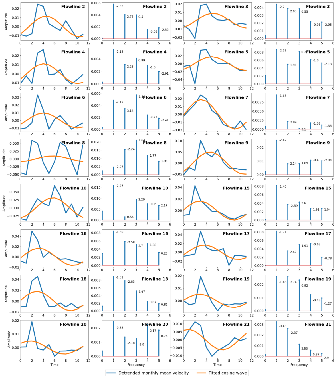
Figure D1 - Discrete Fourier transform outputs. Left hand panels indicate the time domain where time 0 denotes 1st October. Panels show mean monthly ice flow of each outlet glacier (blue; same as Fig. 4) with fitted cosine functions (orange) optimised to the most dominant frequency observed across all outlet glacier time series. Right hand panels indicate the frequency domain, whereby the greatest amplitude associated with each glacier timeseries denotes the most dominant frequency. In the context of the present study, a dominant frequency of 1 denotes one complete seasonal cycle per year. Annotated values indicate the phase associated with each frequency component.
