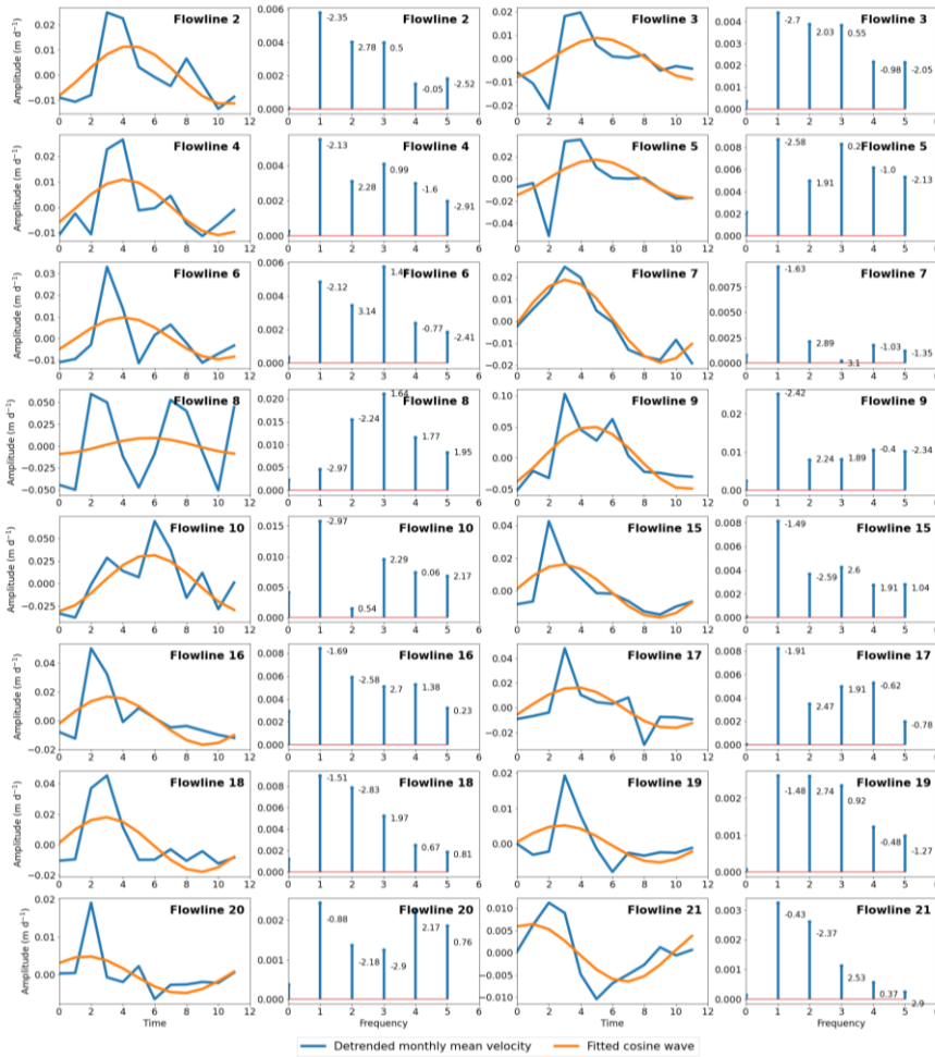
Figure D1 - Discrete Fourier transform outputs. Left hand panels indicate the time domain where time 0 denotes 1st October. Panels show mean monthly ice flow of each outlet glacier (blue; same as Fig. 5) with fitted cosine functions (orange) optimised to the most dominant frequency observed across all outlet glacier time series. Right hand panels indicate the frequency domain, whereby the greatest amplitude associated with each glacier timeseries denotes the most dominant frequency. In the context of the present study, a dominant frequency of 1 denotes one complete seasonal cycle per year. Annotated values indicate the phase associated with each frequency component.
