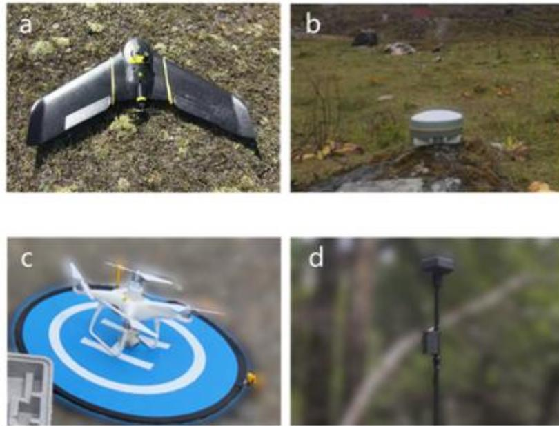
Figure S1: eBee Plus fixed-wing UAV (a), Huaxing A10 GNSS GPS for PPK base station (b), DJI Phantom 4 RTK rotary-wing UAV (c), DJI D-RTK 2 for RTK base station (d).
