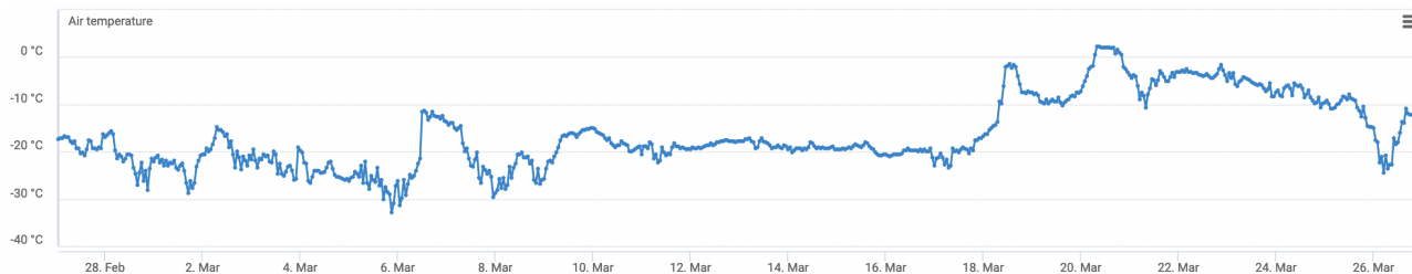
Figure 5. Air temperature recorded during deployment at the Sveagruga weather station (SN99760) located about 2 km west of the experiment. Temperatures remained between -30^{\circ} and -10^{\circ} until March 18th and then remained essentially between -10^{\circ} and -0^{\circ} until the end of deployment, which is consistent with the dynamic of ice thickness shown in figure 7, which exhibits a sharp increase between February 27th and March 16th, and then stabilizes.
