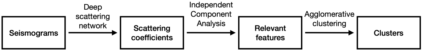
Figure A1. Computing scheme of the Scatseisnet method. The seismograms are fed to a deep scattering network for extracting the scattering coefficients. The most relevant features are extracted from the scattering coefficients with an independent components analysis. Clusters are identified with an agglomerative clustering technique.
