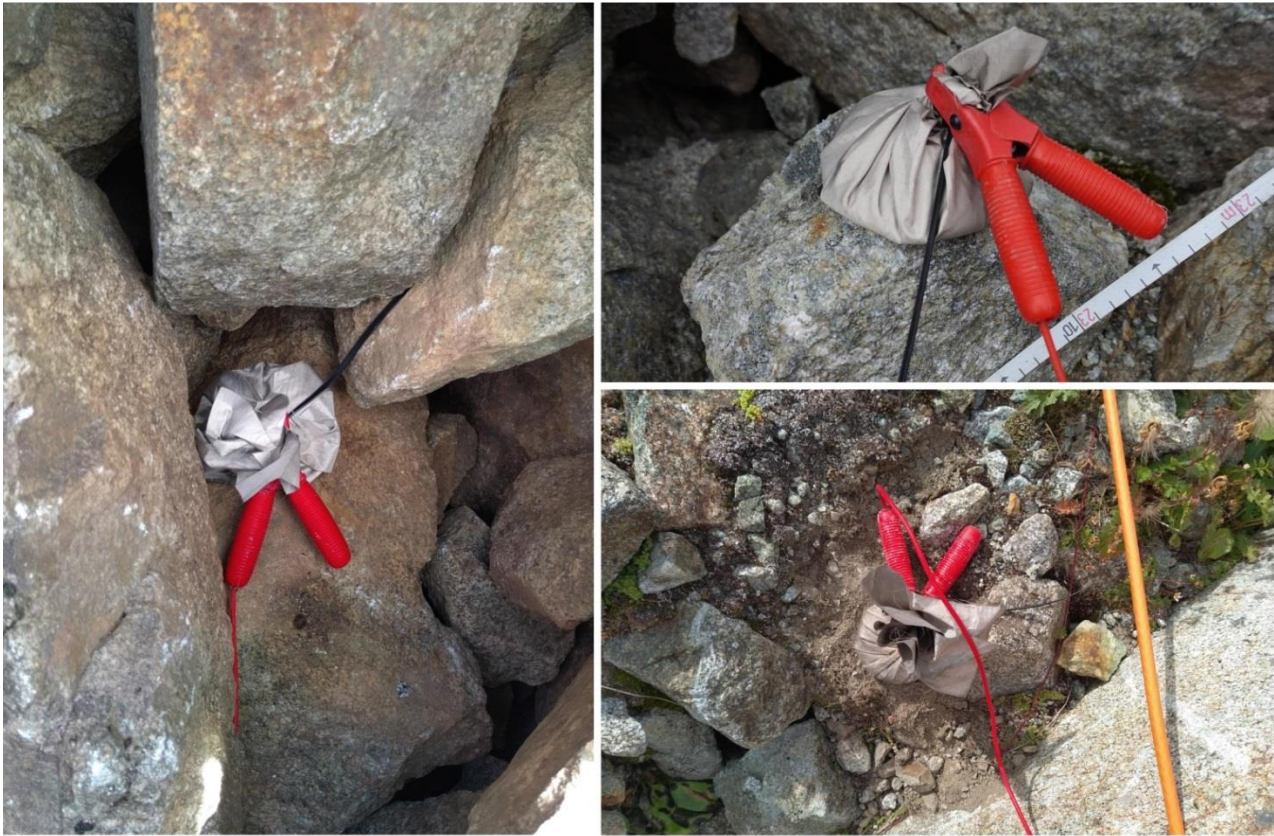
Figure 4: Prototype of the textile electrodes in use. The bag made of conductive textile is filled with 200 g of fine sand. The electrode is connected to the measuring cable by the red clip.
