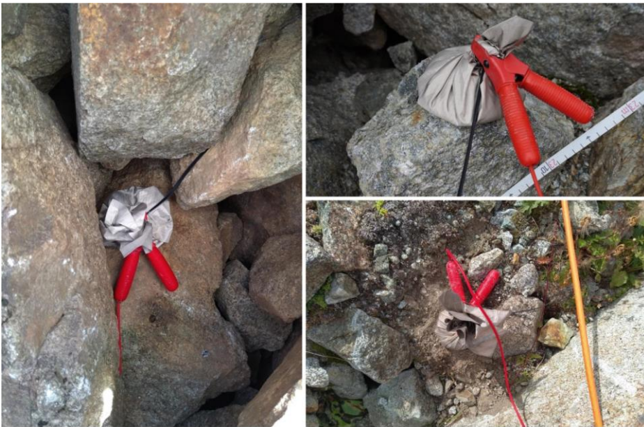
295 Figure 4: Prototype of the textile electrodes in use. The bag made of conductive textile is filled with 200 g of fine sand. The electrode is connected to the measuring cable by the red clip.
