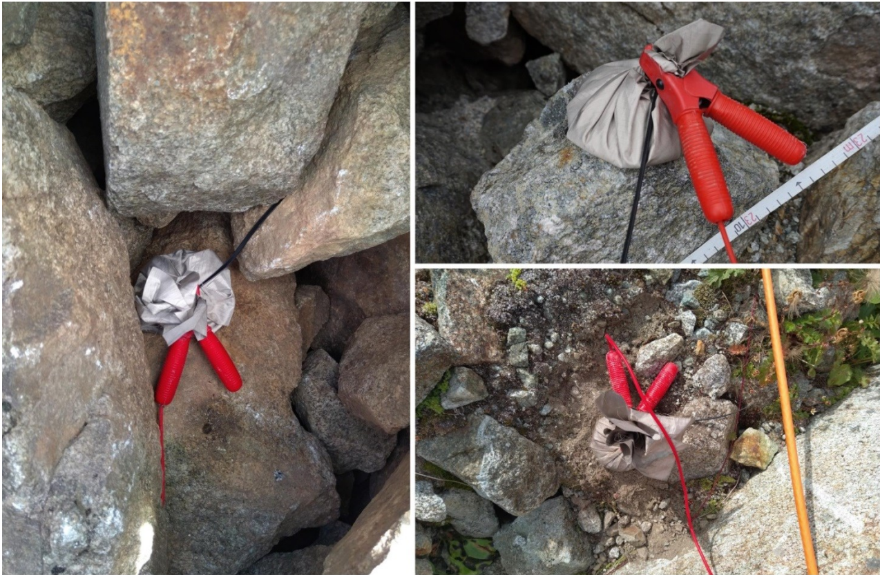
305 Figure 4: Prototype of the textile electrodes in use. The bag made of conductive textile is filled with 200 g of fine sand. The electrode is connected to the measuring cable by the red clip.
