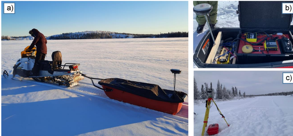
160 Figure 3: (a) The GPR was pulled by a snowmachine. (b) The 1000 MHz sensor was paired with the GPR and an external GNSS rover recorded data simultaneously, to improve the spatial accuracy of the collected transects. (c) A local base station was set up on the lake for GNSS post-processing.
