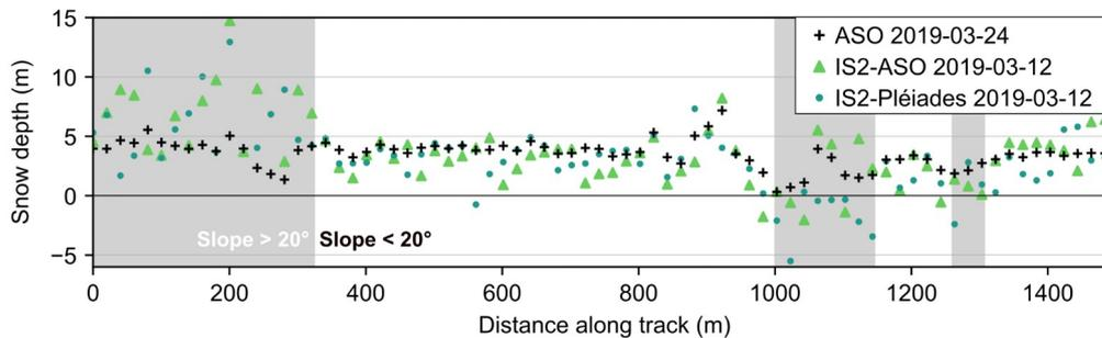
**Figure 4.** Transect of the snow depths on 12 March 2019 derived from ICESat-2 – ASO DTM (green triangles), ICESat-2 – Pléiades DSM (green circles) and on 24 March 2019 by ASO (black cross). Slopes steeper than  $20^\circ$  are shaded as an indication of areas prone to larger errors. This transect is the northernmost of the first beam available on that date (Figure 3a).
