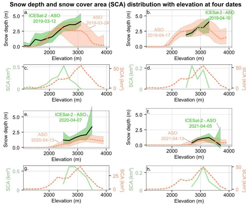
**Figure 6.** Snow depth gradient with elevation (a, b, e, f) from ICESat-2 and ASO snow-off (green) on four selected dates over the three winters of the period and from the closest in time ASO snow depth map (dashed orange). Hypsometry of the snow covered areas (c, d, g, h). The y-axis scale of bottom plots differs to increase the visibility of the smaller surfaces sampled by ICESat-2.
