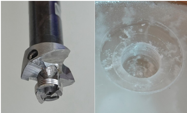
Figure 7: RADIX 20-mm drill bit with 10-mm thread cutting center bit (left). Test drilling in paraffin wax (right).
