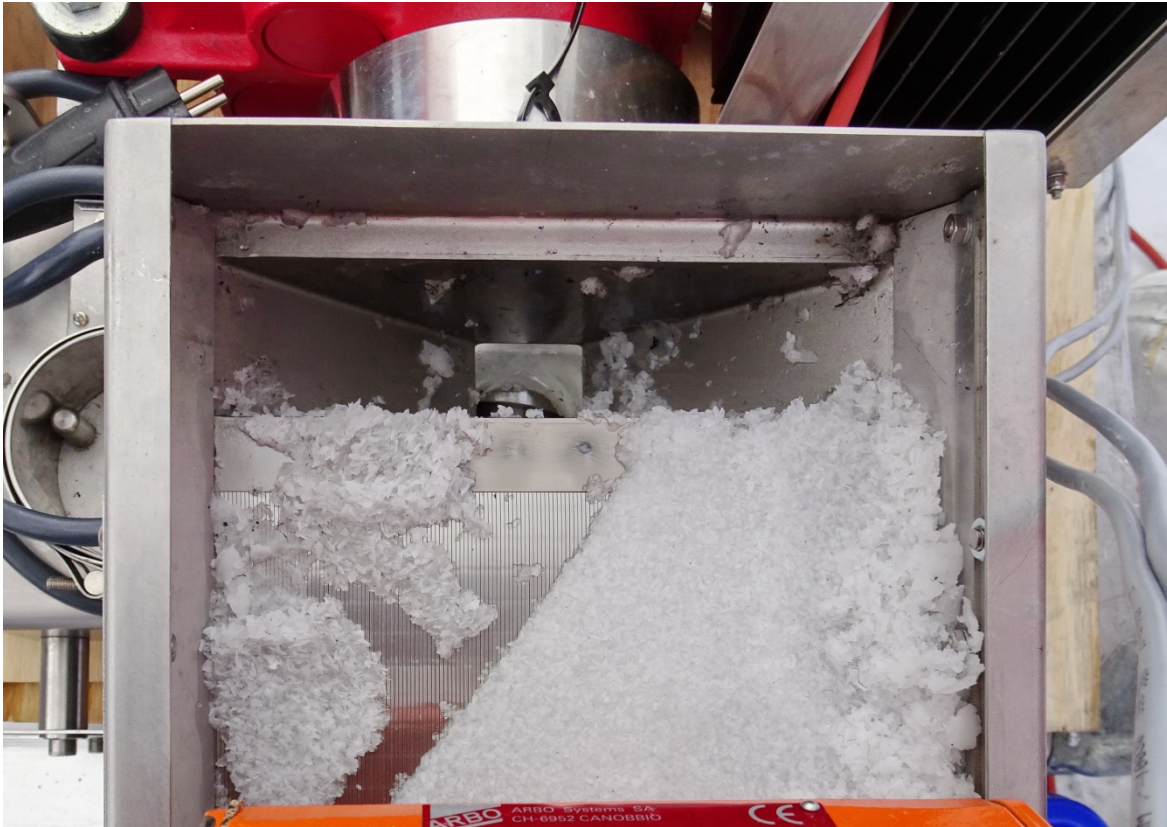
190 Figure 9: Top view of fluid-chips separation on slotted wedge wire screen. The slurry is moving upwards on the vibrating screen and falls into the screw press below.
