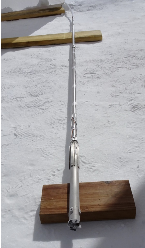
Figure 3: 40-mm firn drill on vacuum line for lifting ice cuttings. All pieces are manufactured in the workshop of the Physics Institute, University of Bern.
