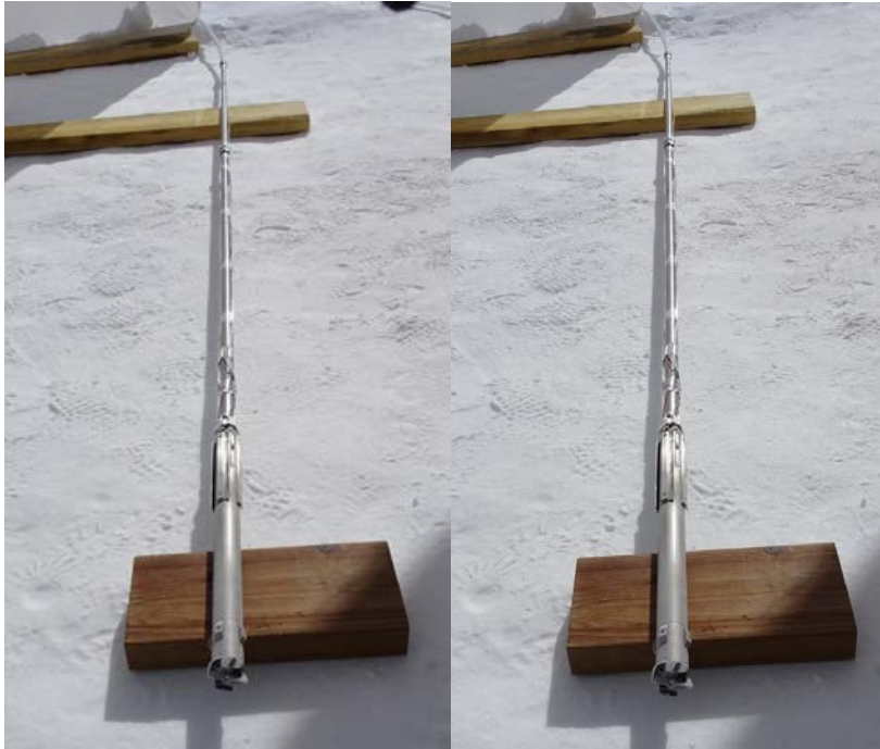
105 Figure 3: 40-mm firn drill on vacuum line for lifting ice cuttings. All pieces are manufactured in the workshop of the Physics Institute, University of Bern.
