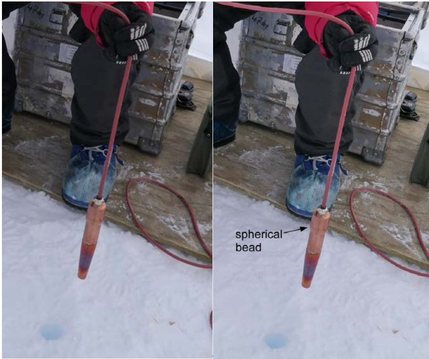
90 Figure 2: Heated copper "plumb bob" for melting and glazing first 6 m of firm hole.
