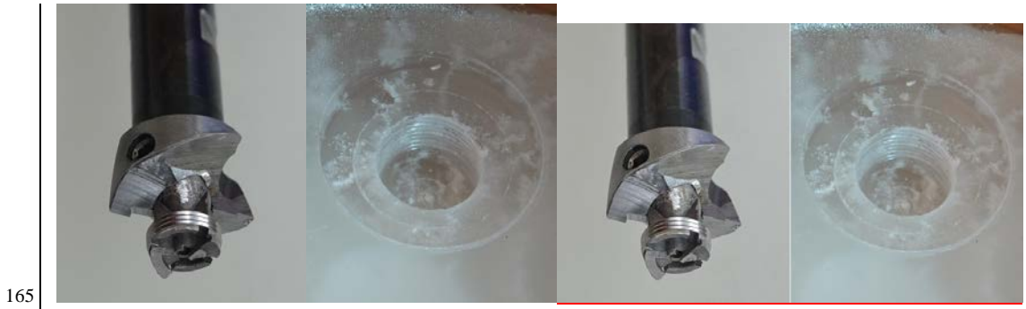
165 Figure 7: RADIX 20-mm drill bit with 10-mm thread cutting center bit (left). Test drilling in paraffin wax (right).
