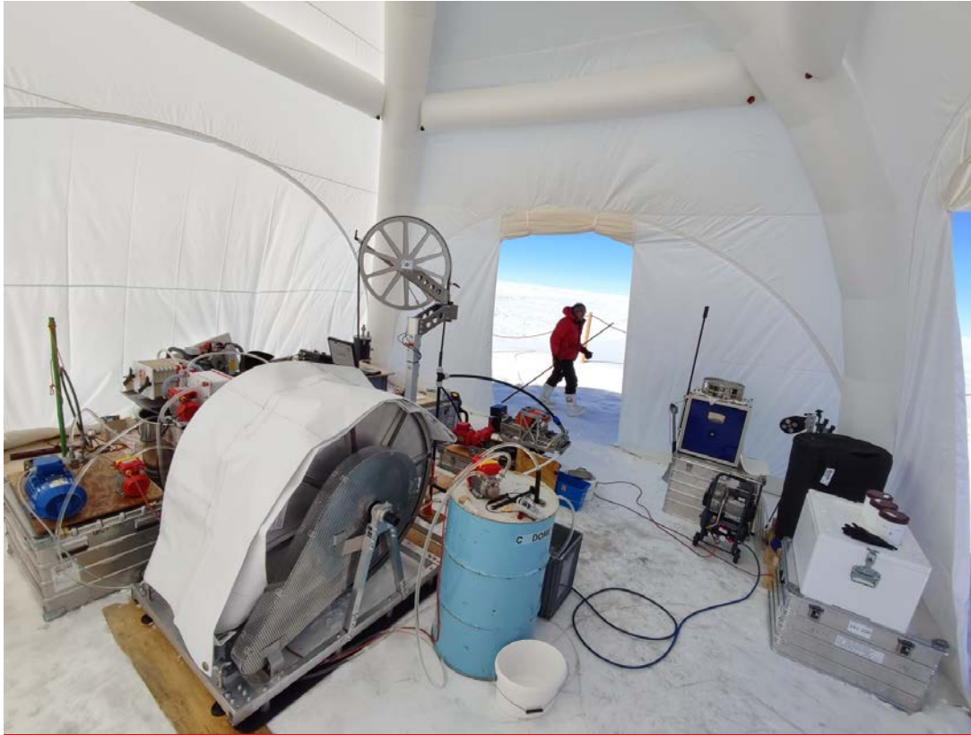
Figure 1: The RADIX system is housed in an inflatable, wind-proof shelter (dimensions: 7m x 7m x 5m) from Axion ( www.axion4event.com ).
