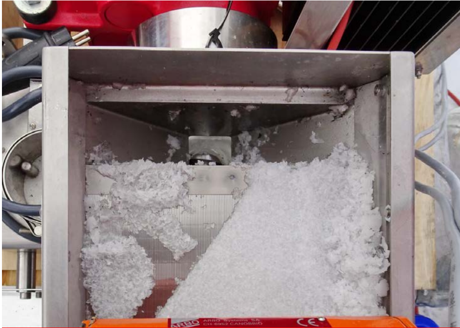
195 Figure 9: Top view of Fluid-chips separation on slotted wedge wire screen. The slurry is moving upwards on the vibrating screen and falls into the screw press below.
