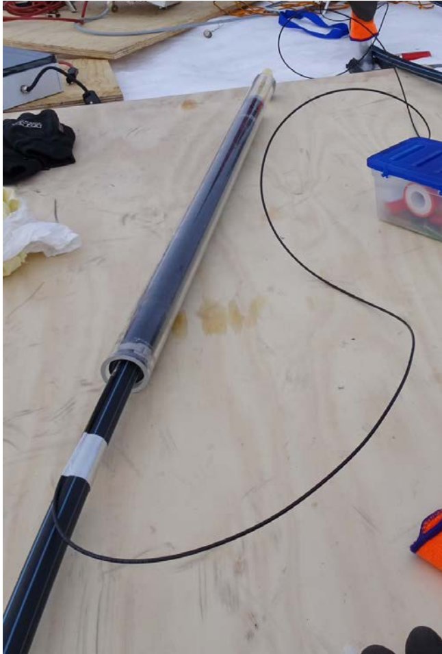
120 Figure 4: Packer inserted into a Plexiglas tube to test inflation. The inner diameter of the tube is identical to the borehole diameter.
