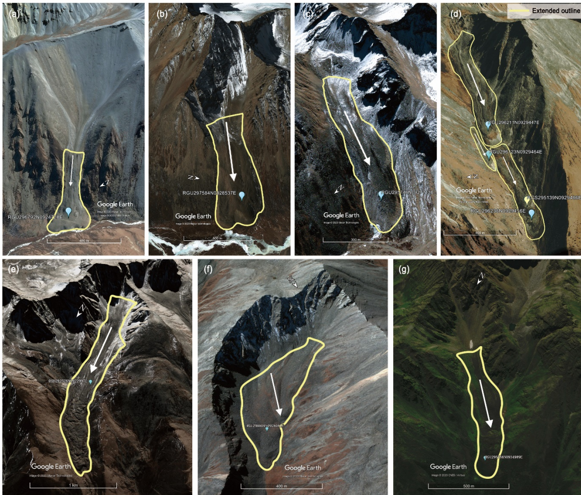
140 Figure 2: Example images of different upslope boundary types of rock glaciers in Guokalariju. (a) a debris-mantled slope-connected rock glacier; (b) a talus-connected rock glacier; (c) a glacier forefield-connected rock glacier; (d) a rock glacier system; (e) an active rock glacier; (f) a transitional rock glacier; (g) a relict rock glacier. Images from ©Google Earth.
