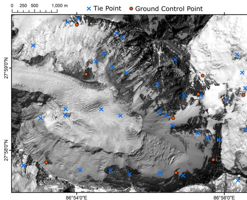
**Resp.Fig.3.** Location of Tie Points and Ground Control Points used during the extraction of the 1984 DEM from three overlapping aerial photographs. Ground Control Points were identified over features which we could confidently assume did not move between the dates of the 1984 aerial photograph acquisition and the 2017 Pléiades scene (i.e. off-glacier terrain).
