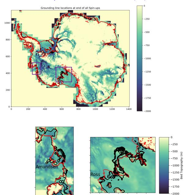
**Fig 1:** Final grounding line positions for all 25 spin-ups (black curves), overlaid on one another. BedMachine observations are overlaid in red. The Amundsen and Ross regions are identified in the top panel. The bottom two panels show these regions in greater detail.
