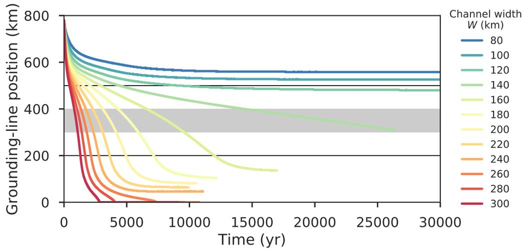
**Figure 5.** Evolution of the centerline grounding-line position (along  $y = 0$ ) of the simulated ice-sheet-shelf system from initialization to equilibration, here exemplarily shown for a variation of the channel width  $W$ . Horizontal black lines denote endpoints of the retrograde section of the bed topography (see Fig. 4B). The characteristic timescale is obtained by averaging the retreat time over the central 100-km long retrograde bed section (grey-shaded region).
