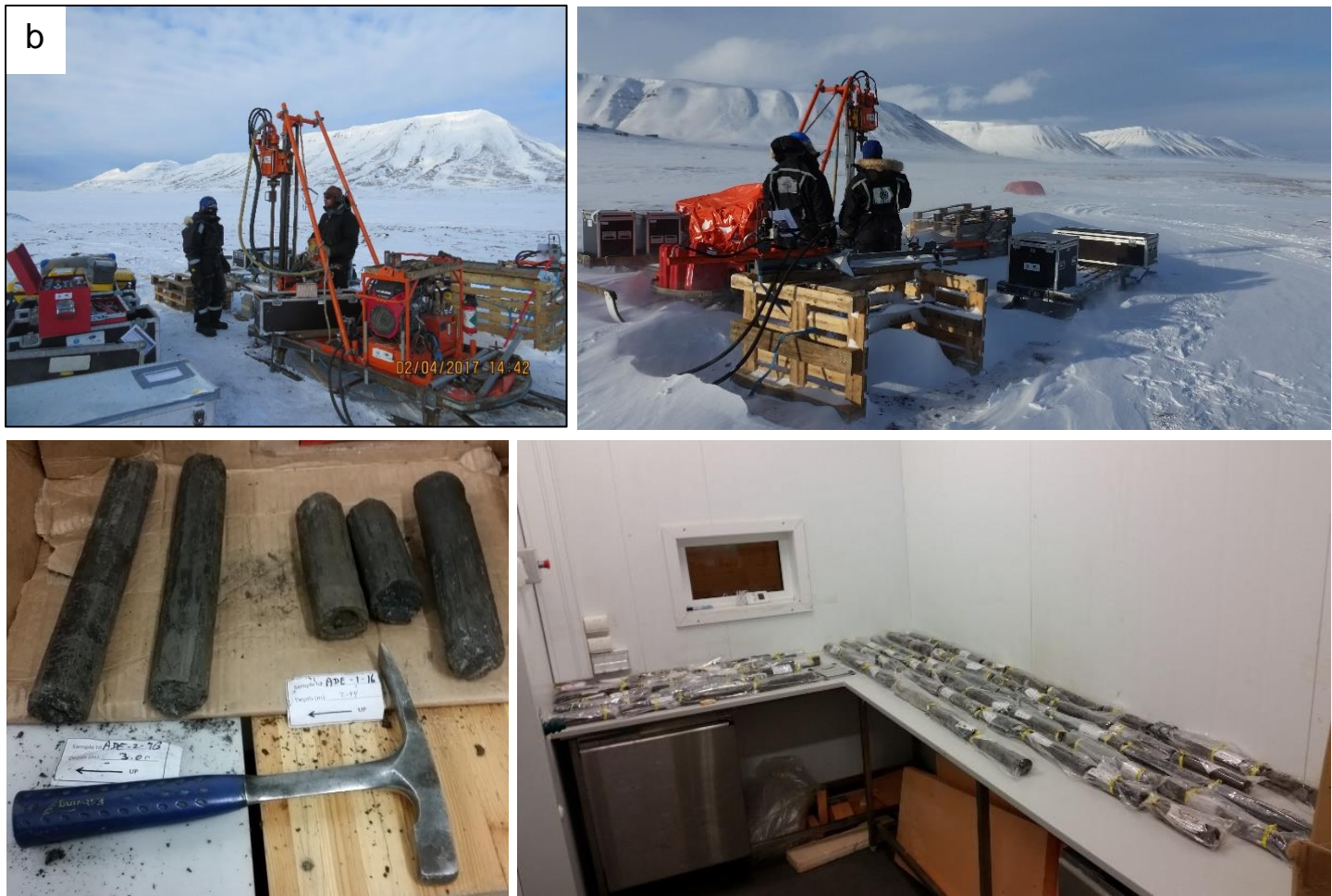
Figure 1. (a) Study site ADE is located at the Adventdalen, Svalbard, on a river terrace. Map provided with courtesy of Norwegian Polar Institute. (b) Drilling at ADE, spring 2017 (top); Cores samples before processing at UNIS cold room lab, (bottom). Photos: Dotan Rotem and Yishai Weinstein.
