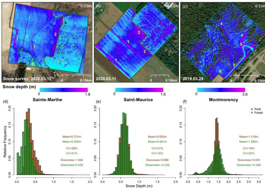
360 **Figure 4.** UAV-lidar derived snow depth maps (grid size 1.4 m) and histograms of snow depth distribution. (a, d) Sainte-Marthe map with snow surveying date and histogram; (b, e) Saint-Maurice map with snow surveying date and histogram. Field and forest areas are demarcated with brown and green colors in snow depth maps respectively. Histograms are derived according to these boundaries. Features 1 to 7 are discussed in the text.
