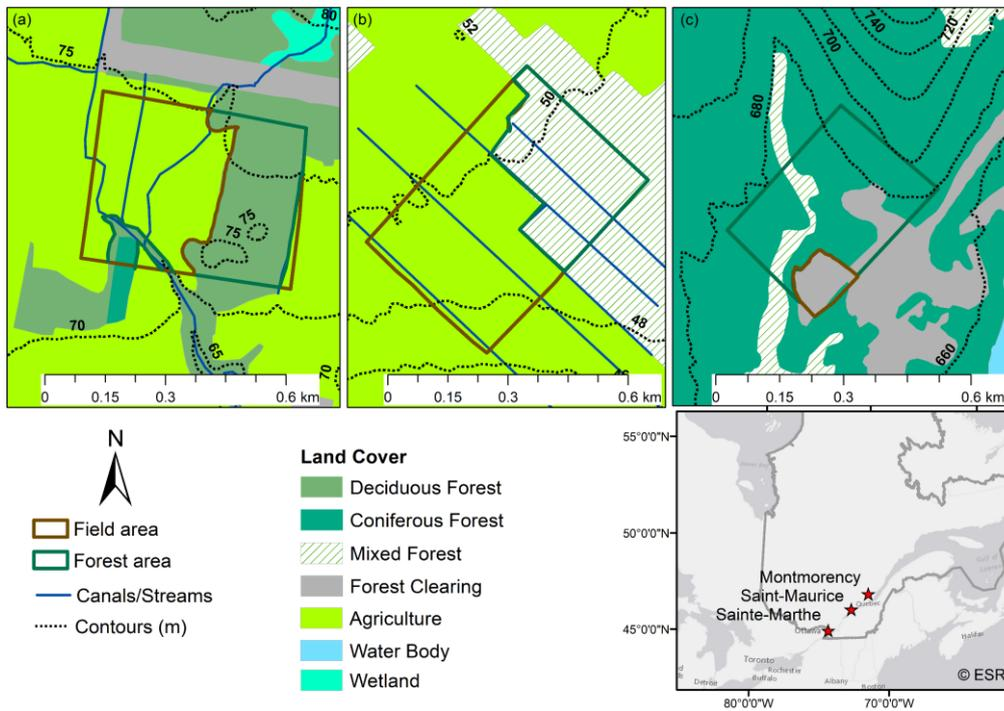
**Figure 1.** Overview of the study sites with lidar survey extents. Field and forest areas within each lidar extent are delineated with brown and green colors, respectively. (a) Sainte-Marthe, (b) Saint-Maurice and (c) Montmorency. Contour intervals intentionally differ between sites for better readability. (Adapted from Dharmadasa et al. (2022))
