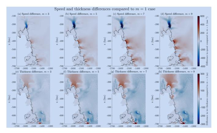
Figure 5. Differences in final speed (panels a-d) and ice thickness (panels e-h) in the *Ice Shelf Removed Branch*, for the Weertman sliding law. All other values of m are compared to the case where m=1. Areas which are not grounded in either case are not shaded as part of each comparison.
