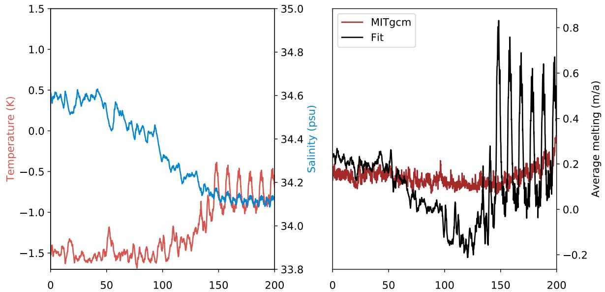
**Figure S5. Testing the Filchner-Ronne Ice Shelf melt relationship.** Left panel: evolution of average ocean temperature and salinity at the depth of the continental shelf in front of the ice shelf in the ocean simulations of the Weddell Sea in Naughten et al. (2021) for the 1 percent CO<sub>2</sub> increase scenario. Right panel: modelled and predicted melt rates using the fitted function from Appendix A1.
