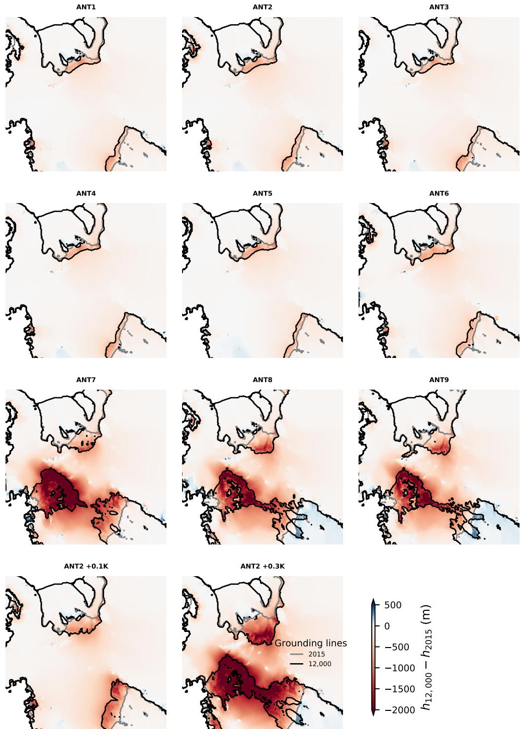
**Figure S3.** Grounding lines and ice thickness changes between year 2015 and after 10,000 of constant present-day climate conditions for all ensemble members in West Antarctica.
