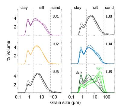
Figure 7. Grain size spectra of lithologic units 1-5 illustrating the similar grain size distributions of sediments in LU1 and LU4, as well as the difference between the dark (less dense) and light (more dense) laminations in LU5.
