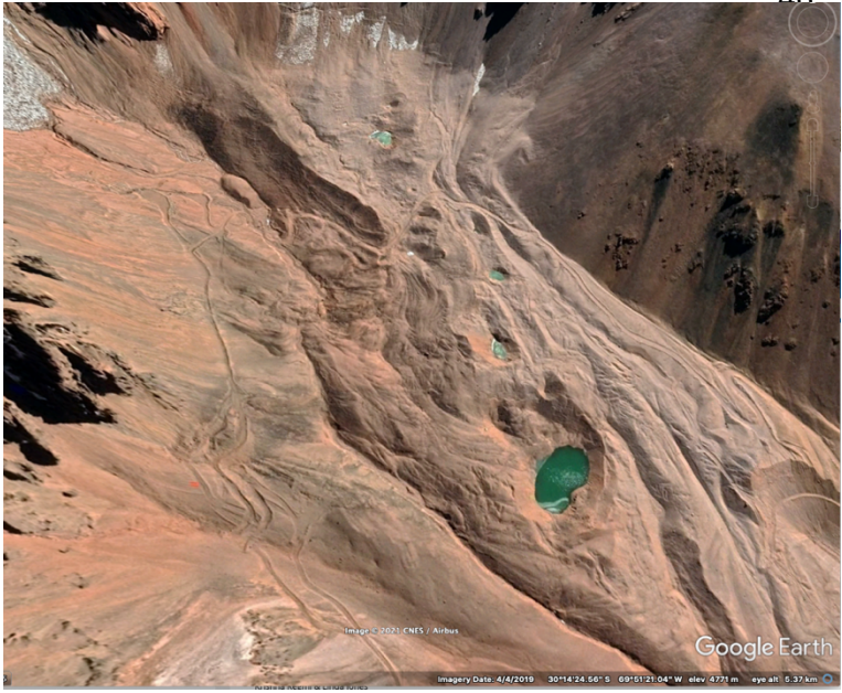
Figure 1. A glacialigenic rock glacier centred on the prominent surface melt pool at [-30.2414,-69.8541] shows ablation of massive, glacier-derived, ice under a debris cover. These melt pools can be traced from the uppermost part of the rock glacier through to near the snout and are persistent over several years of Google Earth imagery. A permafrost (talus-derived) feature would show 'isovolumetric' melting of ice in pore spaces and, thus have rather different water storage capability from a glacier core.
