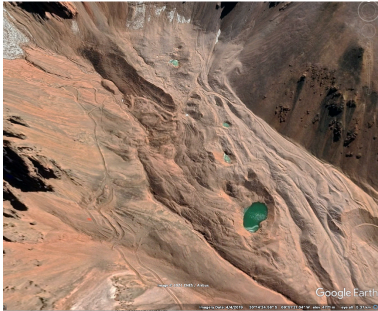
Figure 1. Glacigenic rock glacier located at 30° 14' 29" S, 69° 51' 15" W. © Google Earth/CNES/Airbus. Melt pools, especially at [-30.2414,-69.8541] show ablation of massive, glacier-derived, ice under a debris cover. A permafrost (talus-derived) feature would show 'isovolumetric' melting of ice in pore spaces and thus have rather different water storage capability from a glacier core.
