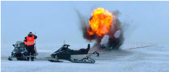
Figure 2 – Photo taken during the 2013 field campaign showing the explosive seismic source. The line of seismic receivers is marked with red poles (Photo: Robert Pfau).
