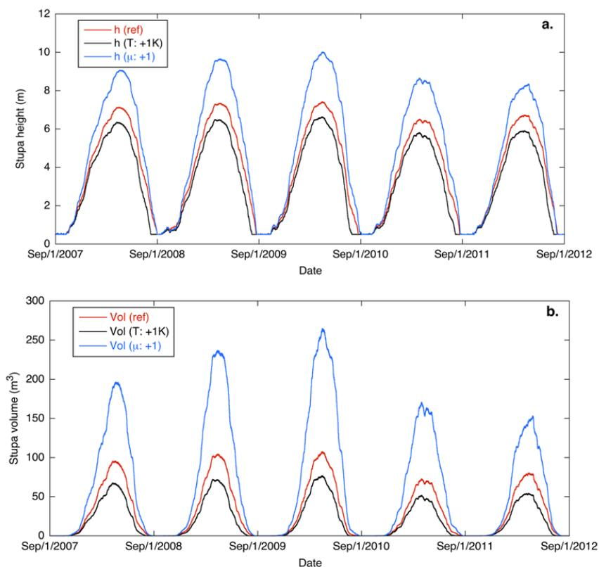
**Figure 3.** Calculated evolution of ice stupa for the case of unlimited water supply for five winters in terms of height (a) and volume (b). The standard run is in red. The blue curve refers to a case with increased exposure parameter, the black curve for a case with a 1 K higher temperature (through the year).
