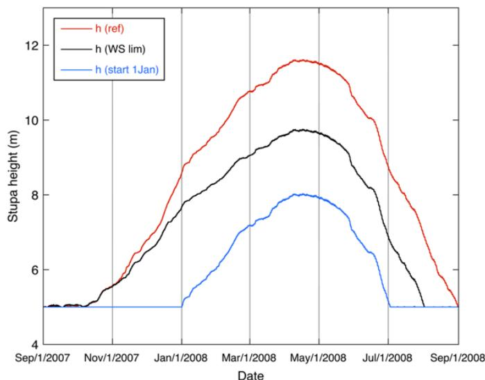
160 **Figure 4.** Stupa height for the case with inner structure (cone) with a height of 5 m. The standard run is in red (with constant albedo). The black curve refers to a case in which the water supply is switched off when the wind speed exceeds 4 m/s. The blue curves refer to a case in which the water supply starts on 1 January.
