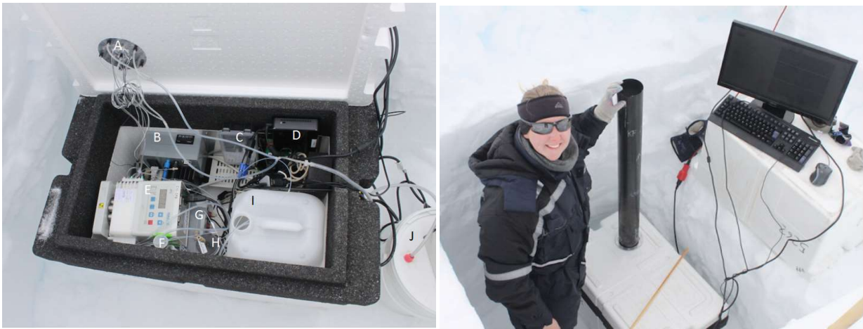
5 Figure 2: Left) An inside look at the LISA box; A) the underside of the melt head, B) melt head temperature regulator, C) temperature PID that stabilizes the inner temperature of the box, D) computer, E) peristaltic pump, F) debubbler, G) fluorescence box (F-box), H) conductivity metre and I) chemical wastewater container, J) container for collecting waste water from the outer section of the melt head located outside the LISA box. Right) LISA box during field work 2017. The snow is collected in the black liner and melted continuously, while data can be observed online on the attached screen.
