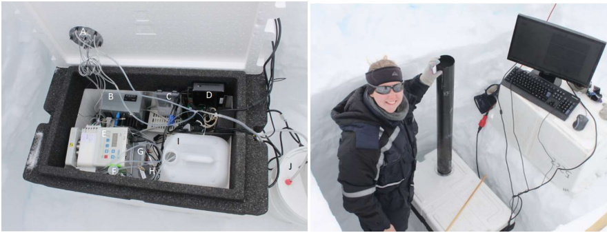
Figure 2: Left) An inside look at the LISA box: A) the underside of the melt head, B) melt head temperature regulator, C) temperature PID that stabilizes the inner temperature of the box, D) computer, E) peristaltic pump, F) debubbler, G) fluorescence box (F-box), H) conductivity metre and I) chemical wastewater container, J) container for collecting waste water from the outer section of the melt head located outside the LISA box. Right) LISA box during field work 2017. The snow is collected in the black liner and melted continuously, while data can be observed online on the attached screen.
