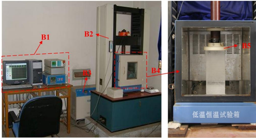
Figure 3: Experiment equipment for the uniaxial compression test: (B1) control system; (B2) loading frame; (B3) refrigerating system; (B4) cryostat container; (B5) pressing plate.
