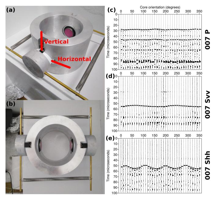
**Figure 4.** (a) Side view of ultrasonic rig with slots for different transducer orientations highlighted. (b) Map view of ultrasonic rig. Transducers are set for vertical vibration. (c) Multiazimuth signal traces using P-wave transducers on sample 007. (d) Multiazimuth signal traces using S-wave transducers set for vertical vibration on sample 007. (e) Multiazimuth signal traces using S-wave transducers set for horizontal vibration on sample 007.
