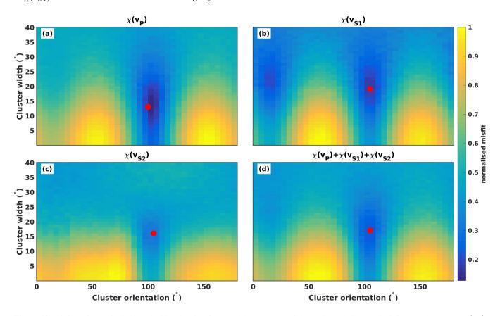
Figure 10. Misfit surfaces of seismic velocities showing fit to model parameters of the Horizontal\_Cluster\_CPO for sample 003: (a)  $\chi(v_P)$  (b)  $\chi(v_{S1})$  (c)  $\chi(v_{S2})$  (d)  $\chi(v_P) + \chi(v_{S1}) + \chi(v_{S2})$
