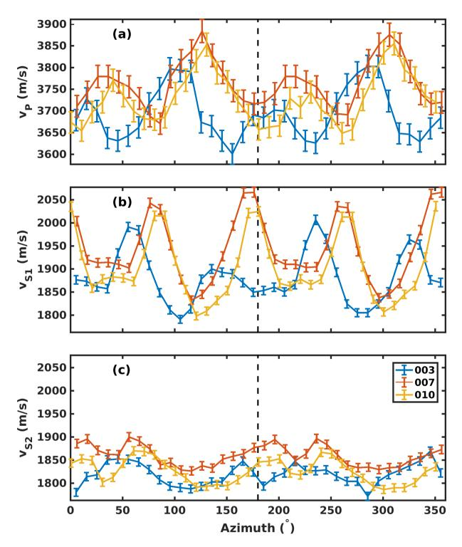
Figure 5. Ultrasonic multiazimuth velocities for different core sections relative to the macroscopic glacier flow direction  $(0^{\circ})$ . (a) P-wave velocity  $v_P$ . The gray-shaded box shows the range of measured vertical ultrasonic  $v_P$ . (b) Fast S-wave velocity  $v_{S1}$ . (c) Slow S-wave velocity  $v_{S2}$ .
