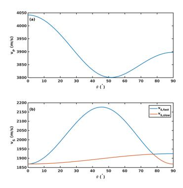
Figure 2. Seismic phase velocities for a single crystal in dependence of angle  $\theta$  to the c-axis, calculated with values for the elastic constants from adiabatic single crystal artificial water ice at  $-16\,^{\circ}$ C from Gammon et al. (1983) using the MTEX toolbox (Mainprice et al., 2011). (a) P-wave velocity  $v_P$  (b) S-wave velocities  $v_S$
