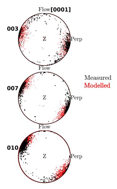
**Figure 11.** Measured (leftblack) and modelled (rightred) CPO geometries. The VSP profile orientations of the "Flow" and "Perp" profiles are labelled. Top row: sample 003, middle row: sample 007, bottom row: sample 010.
