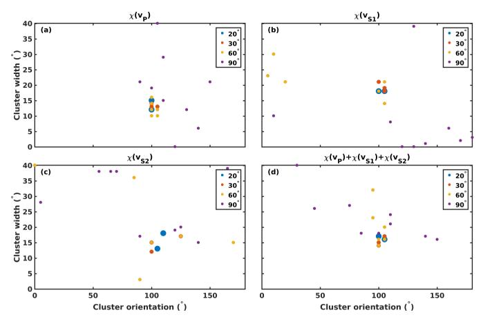
Figure 14. Parameter results using downsampled velocity measurements with azimuthal spacing of  $20^{\circ}$ ,  $30^{\circ}$ ,  $60^{\circ}$  and  $90^{\circ}$  (indicated by symbol size) for sample 003: (a)  $\chi(v_P)$  (b)  $\chi(v_{S1})$  (c)  $\chi(v_{S2})$  (d)  $\chi(v_P) + \chi(v_{S1}) + \chi(v_{S2})$
