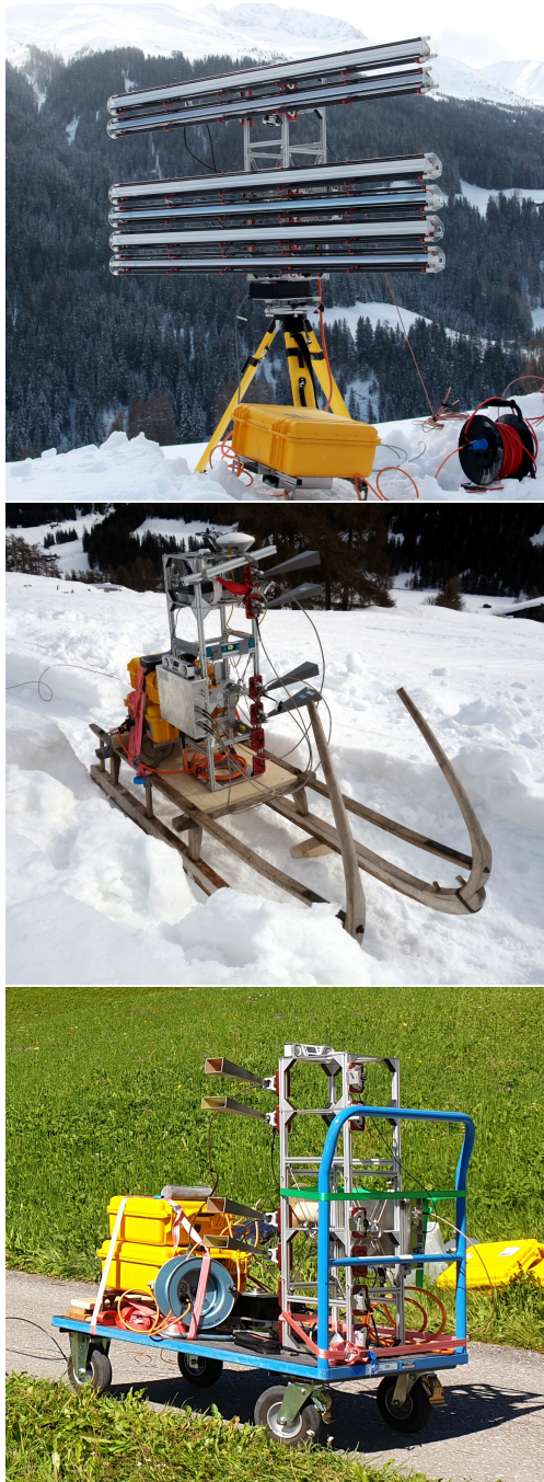
Figure 3. Top: primary KAPRI radar tower (monostatic device) during the ground-based experiment equipped with narrow-beam traveling-wave antennas. Center: secondary KAPRI radar tower (bistatic receiver) equipped with horn antennas and deployed on a "Hornschlitten" sledge in winter. Bottom: secondary KAPRI tower deployed on a wheeled cart in summer.
