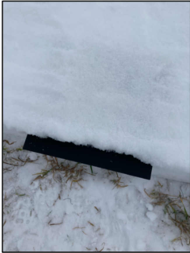
Figure 4. Photograph of the black aluminum panel inserted into the snow pit sidewall approximately 2.5 cm from the surface.
