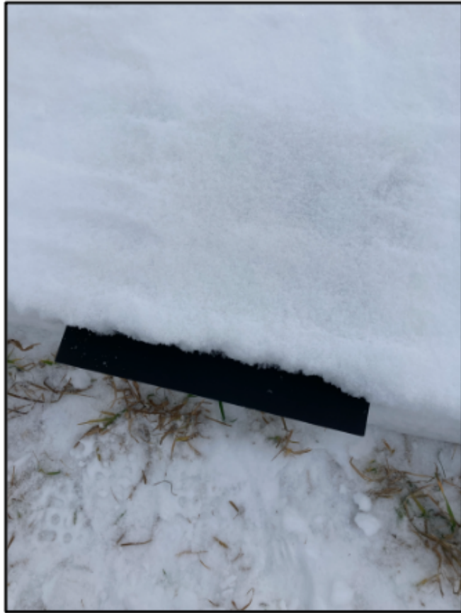
Figure 3. Photograph of the black aluminum panel inserted into the snow pit sidewall approximately 2.5 cm from the surface.
