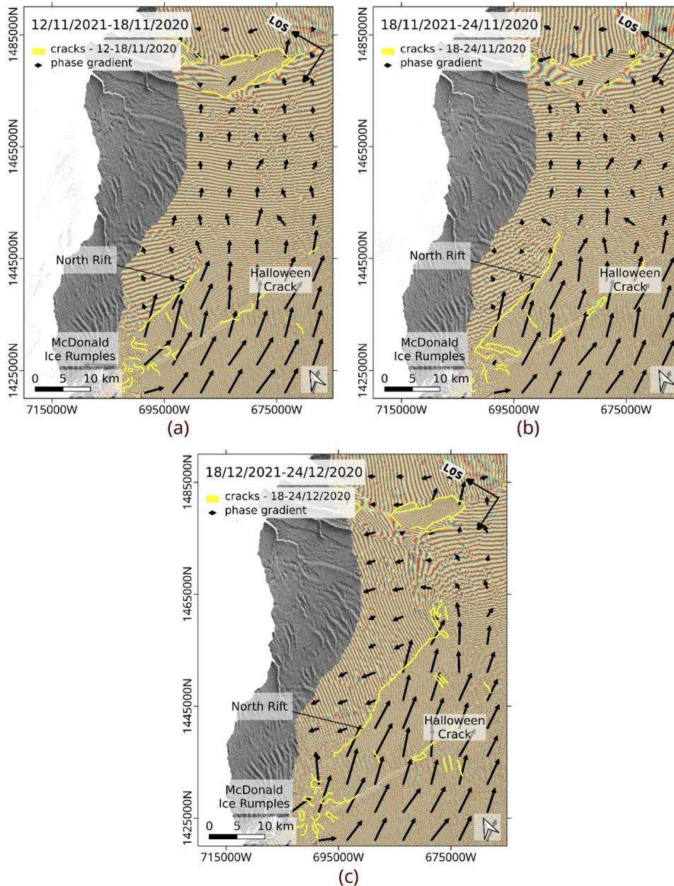
415 **Figure 8: Sentinel-1 repeat-pass interferograms on BIS, overlaid with the cracks delineated from the phase gradient magnitude (yellow lines). The phase gradient is pictured by the vector field. (a) 12–18 November 2020. (b) 18–24 November 2020. (c) 18–24 December 2020. The comparison of the interferograms shows a rapid propagation of the North Rift between 18 and 24 November**
