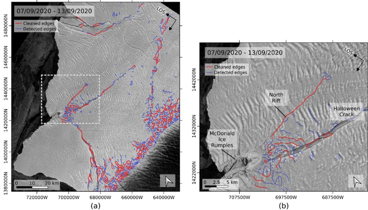
335 **Figure 5: Cracks automatically delineated from the interferogram of 7–13 September 2020. (a) Edge detection results, before (blue) and after cleaning (red) of the small dangles. The Canny edge detection applied to the phase gradient magnitude shown in Fig. 4. (b) Close-up view of (a), whose extent is indicated by the gray dashed frame.**
