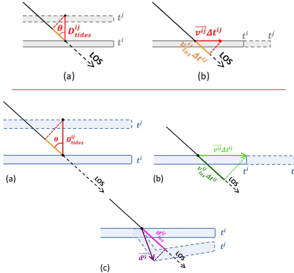
**Figure 2: Displacements and deformations contributing to the interferometric phase over an ice shelf. (a) Change of vertical position caused by tidesal bending. (b) Horizontal ice flow motion. (c) Ice shelf deformation. The ice shelf is represented at times  $t^i$  and  $t^j$  respectively by the continuous and dashed blue-gray lines.**
