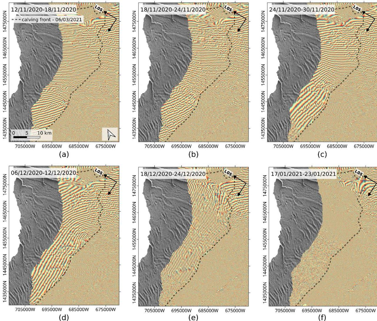
400 **Figure 7: Time series of wrapped repeat-pass interferograms showing the phase ramp variation from one date to another, as the North Rift propagates between November 2020 and January 2021. The black dashed line indicates the full extent of the North Rift, manually delineated from the calving front on 6 March 2021, after the A74 formed.**
