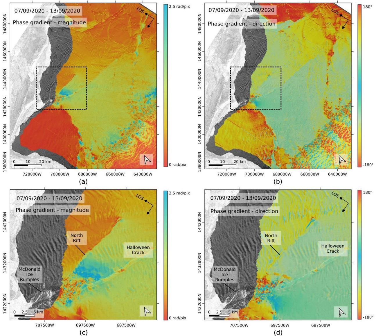
**Figure 4: Phase gradient of the interferogram of 7–13 September 2020 shown in Fig. 1(b). (a) magnitude of the phase gradient. (b) direction of the phase gradient, with angles calculated positive counterclockwise with respect to the horizontal axis. (c) Close-up view of (a), whose extent is indicated by the black dashed frame. (d) Close-up view of (b).**
