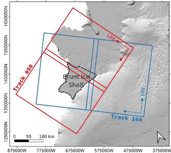
**Figure 6: Sentinel-1 coverage of BIS: track 50 (red) and track 164 (blue). The background is a shaded relief of the REMA DEM (Howat et al., 2019). In IW mode, incidence angles vary from about  $30^\circ$  in the near-range to  $45^\circ$  in the far-range.**
