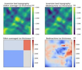
the Bedmachine Antarctica ice thickness (Figure R1) . In this alternate ice thickness dataset, each 50 by 50km region contains only one ice thickness value, which is the average over that region. The
