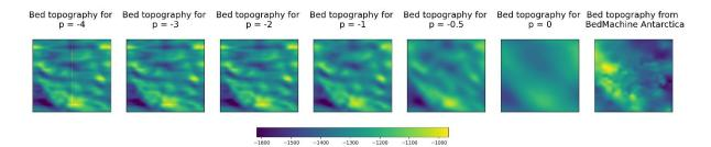
**Figure S3**. Bed topography results of the inversion for the Upper Thwaites region (see Figure 6 for location) with a variety of values of  $p_{filt}$ . Increasing p filters out increasing long wavelengths, and so a value of  $p_{filt} = -2$  is chosen to filter out noisy short wavelengths, while maintaining realistic bed features, as compared to Bedmachine Antarctica (Morlighem et al. 2019)
