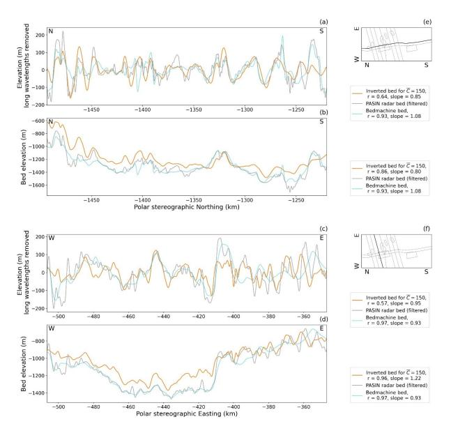
**Figure R3:** The results of the inversion (orange) compared to PASIN radar flight lines (grey) and Bedmachine Antarctica (light blue) for an along flow profile and an across flow profile (locations shown in panels e) and f) respectively). Panels b) and d) show the bed profiles. Panels a) and c) show the results with any Fourier components between 40 and 50km in wavelength progressively damped with a half cosine filter, and any Fourier components over 50km in wavelength removed.
