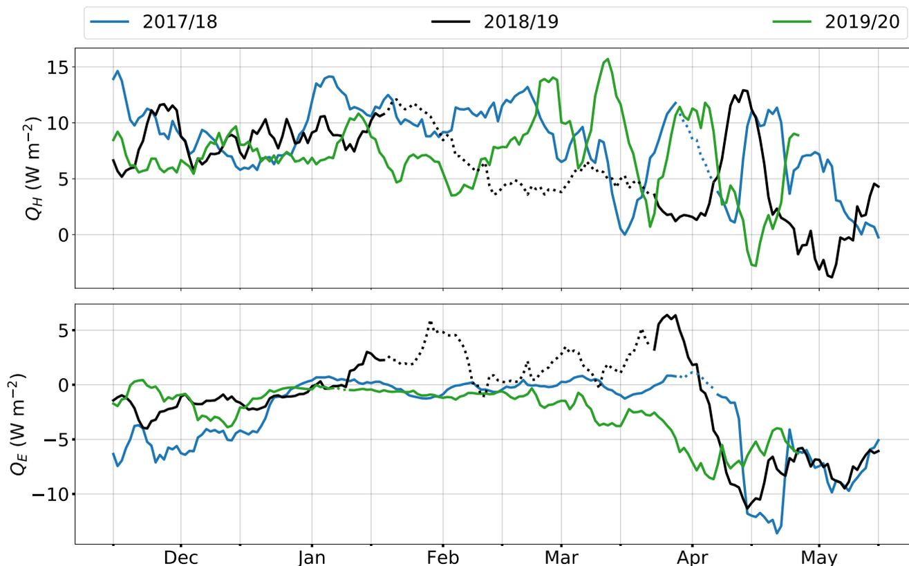
**Figure 4.** Rolling mean of measured daily sensible heat flux ( $Q_H$ ) and latent heat flux ( $Q_E$ ) for the study period. Dotted lines indicate periods of instrument failure which have been gap-filled.
