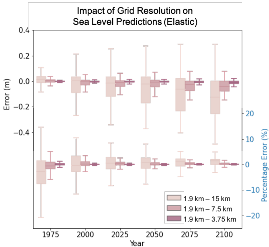
875 Figure 5. Evolution of error in elastic sea-level predictions due to grid resolution from 1950 to 2100 with the 1km input resolution ICE-RD ice model. Box-whisker plots of the error and percent error (see methods) calculated from the difference in predicted sea-level changes from the start of the simulation to the indicated time within 10 km of the grounding line at that time between a simulation with 1.9 km resolution and simulations adopting 15 km (light pink), 7.5 km (medium pink) and 3.75 km (dark pink) grid resolutions. The box represents (from bottom to top) the 25th percentile, median and 75th percentile of the distribution, whilst the whiskers represent the "minimum" (25th percentile - 1.5 x the interquartile range) and "maximum (75th percentile + 1.5 x the interquartile range). Error (m) is the difference between sea-level predictions from the higher - lower resolution simulation. Percentage Error (%) is calculated as 100 * (SL_{1.9km} - SL_{lowres}) / SL_{1.9km} for each grid point. 880
