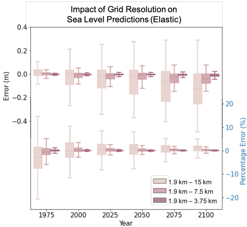
850 Figure 5. Evolution of error in elastic sea level predictions due to grid resolution from 1950 to 2100 with the 1km input resolution ICE-RD ice model. (a) Box-whisker plots of the error and percent error (see methods) calculated from the difference in predicted sea level changes from the start of the simulation to the indicated time within 10 km of the grounding line at that time between a simulation with 1.9 km resolution and simulations adopting 15 km (light pink), 7.5 km (medium pink) and 3.75 km (dark pink) grid 855 resolutions. The box represents (from left to right) the 25th percentile, median and 75th percentile of the distribution, whilst the whiskers represent the "minimum" (25th percentile - 1.5 x the interquartile range) and "maximum (75th percentile - 1.5 x the interquartile range). Error (m) is the difference between sea-level predictions from the higher - lower resolution run. Percentage Error (%) is calculated as 100 * (SL_{1.9km} - SL_{lowres}) / SL_{1.9km} for each grid point.
