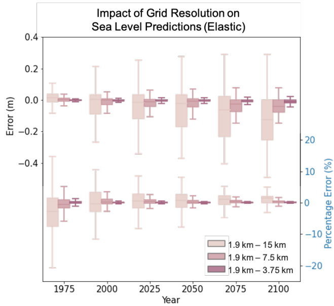
855 Figure 5. Evolution of error in elastic sea level predictions due to grid resolution from 1950 to 2100 with the 1km input resolution ICE-RD ice model. (a) Box-whisker plots of the error and percent error (see methods) calculated from the difference in predicted sea level changes from the start of the simulation to the indicated time within 10 km of the grounding line at that time between a simulation with 1.9 km resolution and simulations adopting 15 km (light pink), 7.5 km (medium pink) and 3.75 km (dark pink) grid resolutions. The box represents (from left to right) the 25th percentile, median and 75th percentile of the distribution, whilst the whiskers represent the "minimum" (25th percentile - 1.5 x the interquartile range) and "maximum (75th percentile + 1.5 x the 860 interquartile range). Error (m) is the difference between sea-level predictions from the higher - lower resolution run. Percentage Error (%) is calculated as 100 * (SL_{1.9km} - SL_{lowres}) / SL_{1.9km} for each grid point.
