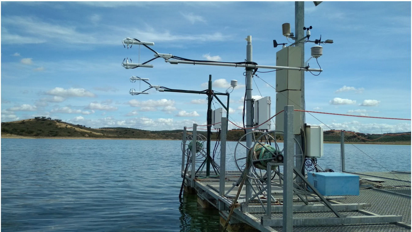
Figure A1: The instruments installed in Alqueva reservoir (Portugal) for the intercalibration. The left instrument belongs to the Institute of Earth Sciences, and the instrument on the right belongs to the Finnish Meteorological Institute.
