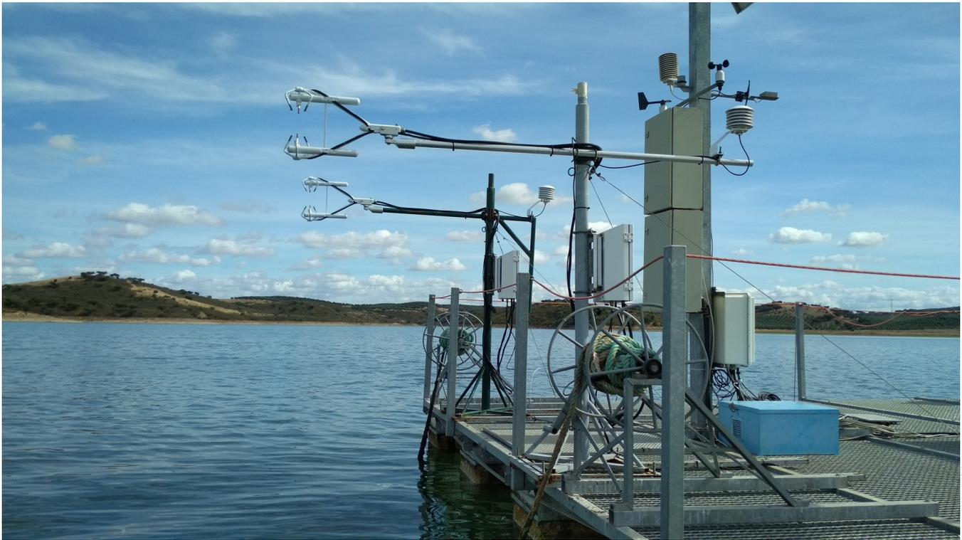
**Figure A1: The instruments installed in Alqueva reservoir (Portugal) for the intercalibration. The left instrument belongs to the**
