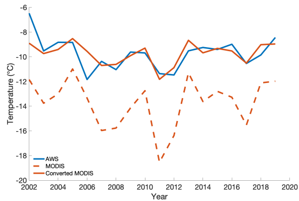
Figure 12. AWS temperatures, MODIS LSTs, and MODIS LSTs converted to air temperatures at Divide. Unconverted MODIS LSTs (dashed orange line) show a prominent offset from AWS measurements, but overall agreement in years of high vs. low temperatures. MODIS LSTs converted to air temperatures by applying a simple linear regression (solid orange line) show much closer agreement with AWS temperatures (solid blue line). All temperatures are mean annual values.
